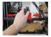
If you are able to wiggle your extruder, the eccentric spacers on the bottom of the extruder will need to be adjusted.
