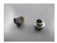
Eccentric spacers are used to adjust the amount of pressure the V-slot wheels put on the V-slot rails. The hole drilled through the center is actually offset so the when adjusted, it will change the position of the wheels. Over time you may have to adjust these wheels if your extruder or aluminum bed feels loose. Most of our spacers can be adjusted with an 8mm wrench. Older versions, you will need a 10mm wrench.
