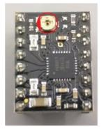
There is a flat spot on the potentiometer. We use this a visual indication to determine how much to adjust the potentiometer.
