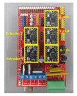
The first step will be to identify the correct stepper driver to adjust depending on the axis that is layer shifting. If you are experiencing layer shifting, it will most likely be in either the x or y axis. But adjusting the z-axis can be used if your printer is having trouble raising the xaxis arm.
