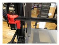
After everything is loose, you want to make sure the x-axis arm is level to the bed. This can be done with a ruler. Simple measure the distance between the bed and xaxis arm. If one side is higher or lower, you can manually turn one of the lead screws to make sure both side are equal distances away from the bed.
