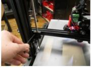
After the auto home function has finished, you want make sure the lead screws are point straight up. You will also take this time to tighten the nutblock on the x-axis arm.
