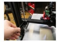
You will start by loosening the bolts on the nutsblocks and the lead screw holder
