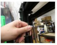
Once the x-axis arm is at the top of the frame, you can tighten the lead screw holders. And your lead screws are now aligned!
