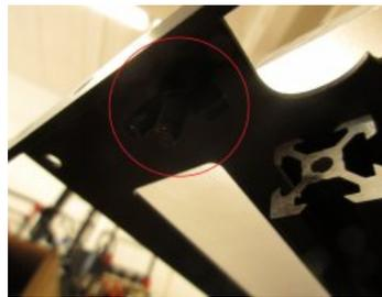
The acrylic bed has 4 mounting bolts holding it in place. Under the aluminum bed, there are wingnuts and split lock washers used to help tighten the acrylic to the aluminum bed.
