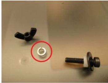
If you do fully remove the hardware, make sure to put the split lock washer in between the wing nut and the aluminum bed. Otherwise the wingnut may come loose and let the acrylic bed shift during printing.
