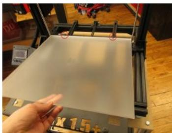
When replacing the acrylic, place the back end of the piece in first. Make sure the washers are sitting on top of the acrylic.
