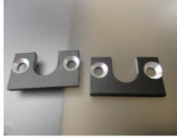
After the J-head hotends have been disconnected, you are going to need to remove the M5x40mm Bolts holding them in place. Make sure to save aluminum plate at the top of the J-head hotends. These plates will be needed to install the E3D hotends.
