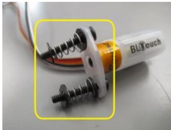
After you have removed the bracket, make sure to save all hardware used to mount the BLTouch to the bracket. You will need these to mount the BLTouch to the new bracket that was sent with the kit. Notice that you need to have the spring sandwiched between the two washers.
