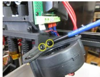
You are going to start with removing the LED Light cover on your gMax printer. Followed by removing the fan shroud that is currently installed.
