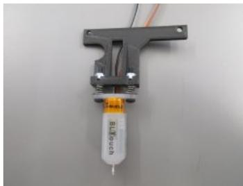
The new bracket has locknuts installed to help prevent the BLTouch from losing its height. You are going to want to tighten the screws down until there is about 1/4" gap between the top of the BLTouch and the bottom of the bracket.
