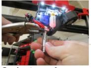
With the old nozzle removed, you can hold onto the socket to quickly screw the new nozzle into place. Once it is snug, make sure the hotend is still at 200c so that you can hot tighten the nozzle to the heater block. This will help prevent nozzle from coming loose over time.
