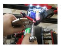
After the E3D has reached temperature, you can use the pliers to hold onto the heater block. With the 7mm socket, start to loosen it and keep turning to remove all the way. Be careful at this point as the heater block and nozzle are VERY hot and can burn you if touched.
