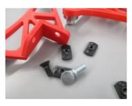
The first step to install the filament spool brackets will be to remove the mounting hardware. Due to the stabilizing brackets, it is not possible to just slide the brackets onto the 80/20 rail.
