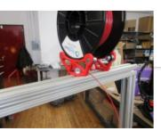
We recommend the filament spool be placed so it unspools from the bottom to prevent the spool from falling off during a print
