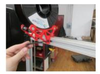
While holding your spool of filament up on the tightened bracket, slide the second bracket into place to support the other side of the filament spool. Tighten the thumb screw to hold it into place. Then tighten the bolt on the back of the bracket.
