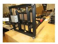
Once the plate is installed, reinstall the aluminum bed and tilt the printer back. You can support the top of the printer with an old filament box. Attach the Y-axis plate to the aluminum bed with the (2) M5x10mm low profile bolts and the tnuts that should be installed on the aluminum bed frame.
