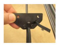
Insert remaining belt into vertical slot on metal plate. To tighten the belt in the future, simply loosed the double tnut and pull belt tight.
