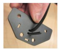
Insert the GT2 belt in the top hole of the metal plate with ribbed side down.
