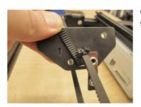
Once belt has been run through rear pulley and motor bracket, insert belt into lower slot of the metal plate. Pull excess belt up towards top of bracket.
