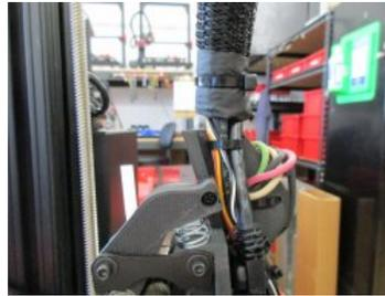
At this point, you will need to run the long BLTouch wires to the electronics box. You will need to either clip the zip ties and run the wires inside of the tech flex, or you can simply zip tie the wires to outside of the wiring bundle.
