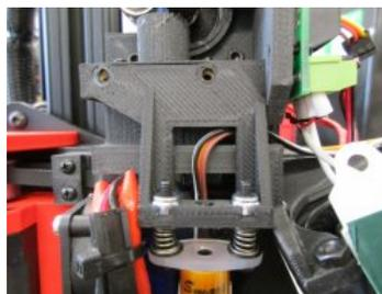
With the LED cover off, you can feed the BLTouch wires through the slot on the extruder. Make sure to feed the wires straight up when placing the BLTouch. Otherwise, the wires can get pinched between the bracket and the extruder.
