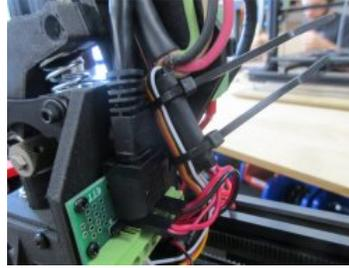
To secure the wires in place, wrap a piece of tape around the wires. Flip the connection and zip tie together to help prevent wires from being pulled apart.
