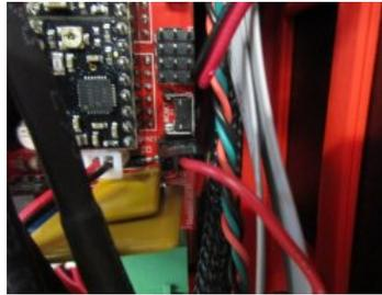
You will then use the pliers to remove the 5v jumper on the electronics board. The single red wire on the BLTouch power wire will then be installed in place of the jumper. Make sure the single red wire lines up with the center pin.
