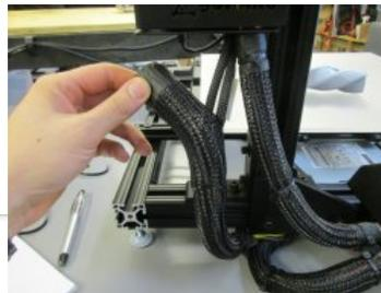
Next replace the rear cover on the LCD housing and replace the tech flex. If you have spare zip ties, you can secure the tech flex again.
