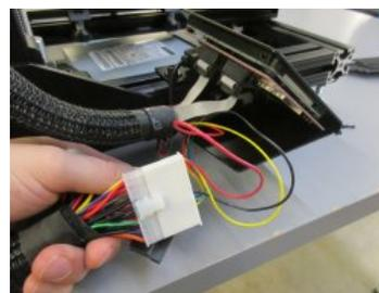
Next you will need to remove the 4 screws holding the rear cover onto the LCD housing. With that removed, you will disconnect the rest of the wires at the 24 pin connector. Be careful not to pull on this connector to hard, or you can disconnect the power button for your printer.
