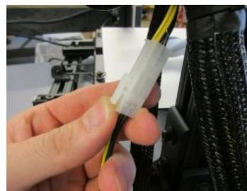
With the zip ties clipped, you can remove the tech flex covering the wires. Next you disconnect the 12v power at the connector shown.
