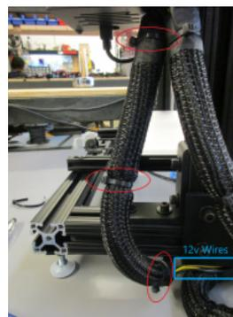
To replace the power supply on your gMax 3D printer, you will first need to remove the tech flex around the 12v wires, and free up the other power supply wire bundle. Clip the large and medium zip ties shown. You will only need to clip the medium zip ties on the wire bundle holding the 12v wires.
