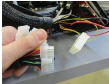
Now you can reconnect 12v wires and the 24pin connector.
