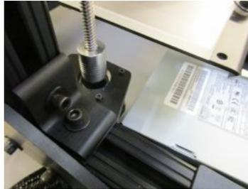
When installing the new power supply, start with the t-nut and bolt closed to the power supply body. You can use a smaller allen key to hold the t-nut in place during this process. Before tightening the bolts, push the power supply as far back as it will go.
