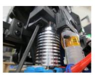
With dual extruders, you will want to remove the active cooling fan to be able to access the E3D mounting screws. It is recommended to unplug the fan from the quick disconnect when removing it. Otherwise you run the risk of jerking the wires out of the active cooling fan and will need to replace it.
