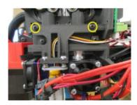
Next you will need to remove the fan shroud to be able to loosen the bolts holding the E3D in place. You can remove the BLTouch as well if you would like a little more room.
