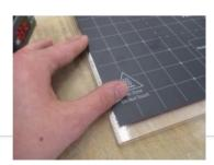
Now you can place the sheet of BuildTak on your heated bed. Make sure to line the edges of the BuildTak up with the edges of the heated pad on the opposite side.
