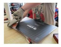
Once the heated bed has reached 90c, you will want to put on the glove to prevent burning yourself, as you will be handling the hot bed. You can then use the razor blade to lift up one of the corners of the BuildTak. Once you get the corner up, you can grab the BuildTak with your hand and start pulling it off of the heated bed. The key to removing the sheet of BuildTak is slow and steady. Trying to rush could result
