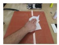
After your heated bed has cooled down, you will want to spray the glass surface with the Rapid Tac and wipe clean. This product is used as both a cleaner and application fluid.
