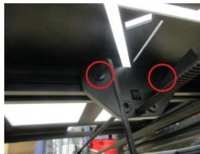
To start, you will want to remove the endcaps on the back of the v-slot rails. Then disconnect the Y-axis bed plate and slide the entire bed off the back of the printer.
