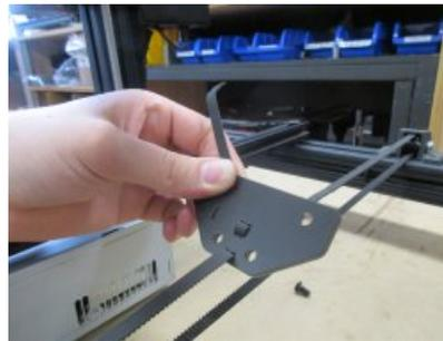
Now you will insert the other end of the GT2 belt through the bottom belt slot on the bed plate. You will want to pull this tight to remove any excess slack in the belt.
