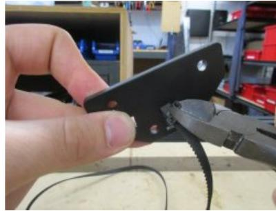
You will then need to clip the zip ties holding the other end of the GT2 belt in place. Once clipped, you can pull the GT2 belt out of the Y-axis plate. You can now remove the old belt from the pulley and drive gear.
