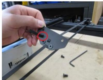
While holding the belt tight, you will need to reattach the double t-nut to hold the belt in place. Then insert the excess belt through the side belt slot on the bed plate to prevent it from dragging on the GT2 belt and causing skipping.
