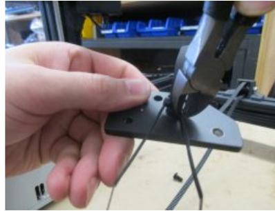
At this point, you will use the two zip ties to hold the GT2 belt together. With the teeth of the belt facing each other, it will lock the GT2 belt in place and prevent slipping. You will then want to clip the excess zip tie.
