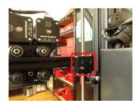
You can find the nutblocks on the back side of the x-axis arm where the LEAD screw meets
