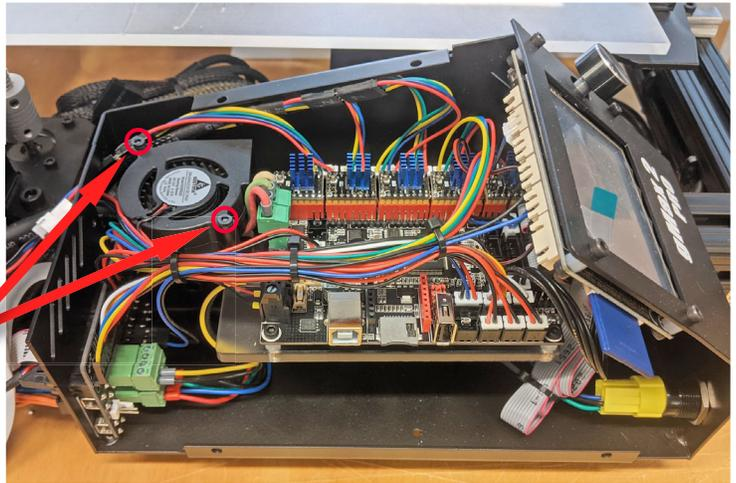
3. Install (3) M6x12mm socket head bolts w/ M6 washers to connect the case to the frame in existing tnuts from old case.
