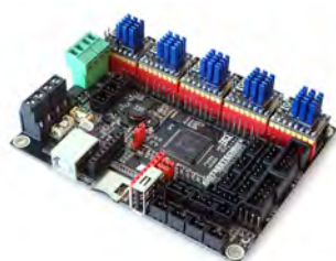
32 Bit Electronics with Silent TMC2130 Stepper Drivers
